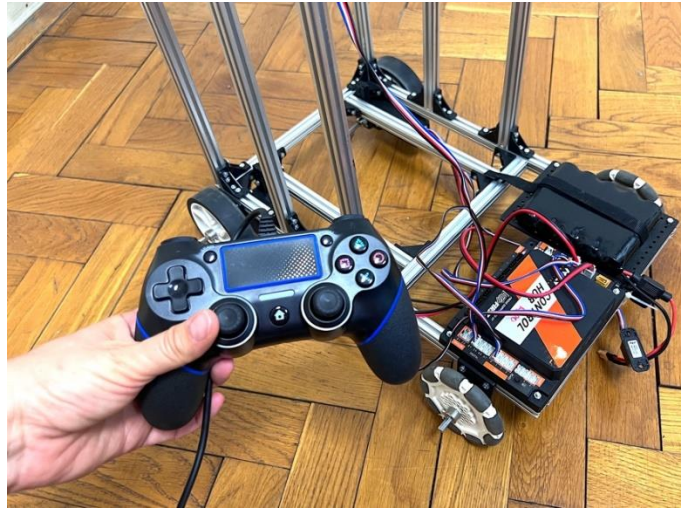
Figure 16. Robot controlled via remote controller.
