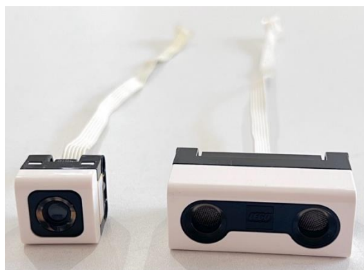
Figure 6. Color and ultrasonic sensor for Lego Spike Prime robots.
