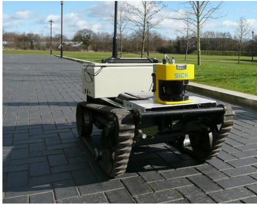
Figure 7. Mobile robots are equipped with a LIDAR sensor, allowing it to map the surrounding area and avoid obstacles [8].
