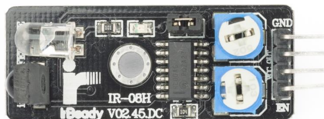
Figure 5. Infrared sensor for detecting obstacles or black line.
