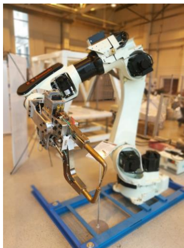
Figure 1. Spot welding robot [4].
